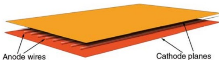
Fig. 4.17 Schematic representation of a multi-wire proportional chamber (MWPC). The cathode planes are at ground potential and the anode wires are at a large positive voltage, typically 3000 V. Each anode wire is equipped with its own amplifier and readout electronics. If a charged particle crosses perpendicularly to the plane of the detector, the wire nearest to the crossing point will have a signal
